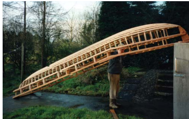
Jarlath carrying the framework of an Aran Island currach – one of the many boats he has built over the years
